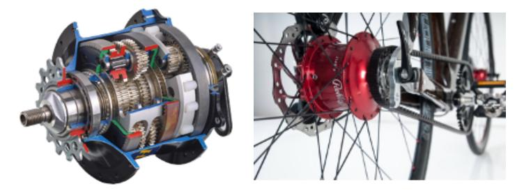
I mentioned maintenance. Yes, even the Ruhloff needs it. So, at every 3,000 miles one must perform a relatively straight forward oil change. It requires about to 10 minutes to drain and replenish the oil. The lifespan is well over 60,000 miles.
